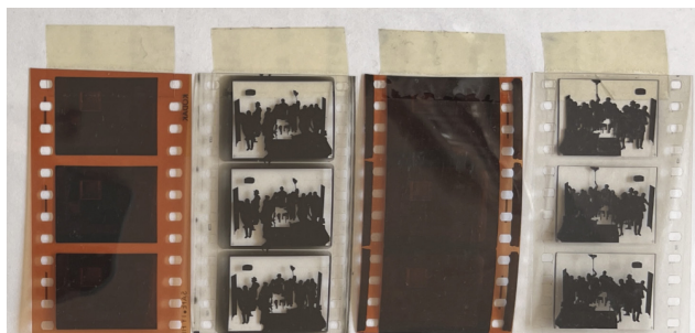
Fig. 11: Live-action footage — intermediate film stock, mask for background-high contrast, background exposition, black and white copy for sound. Source: Zbigniew Weresa. Photo: Agata Hofelmajer-Roś
